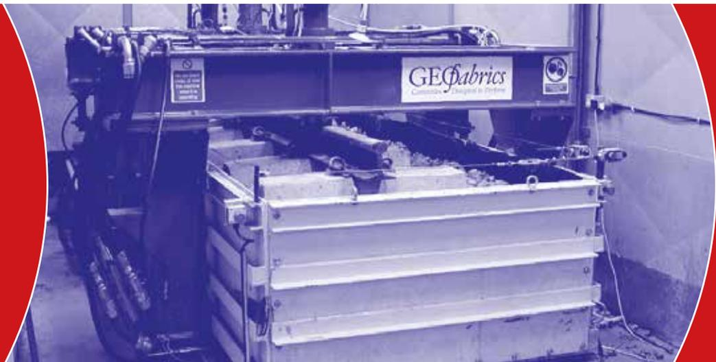
TrackTex has been tested to conditions simulating mud pumping failure in a full-scale purpose-built test facility. The completed facility comprised a 4.5m x 1.5m tank, deep enough to accommodate 200mm of subgrade, 300mm of ballast, 7 half width sleepers (ties) and a length of rail. This state of the art facility allows materials to be tested to the most extreme conditions found in trackbed.
