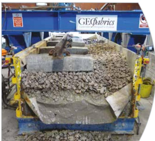
Failed pumping test using standard geotextile separator
