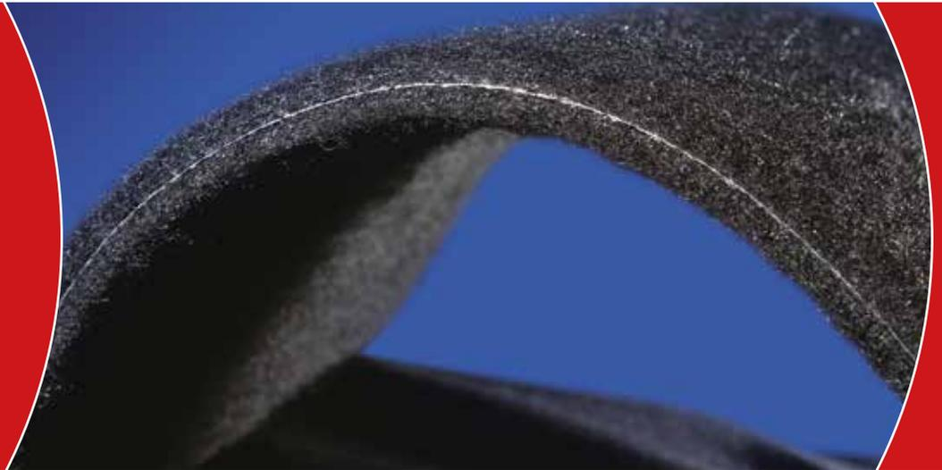
TrackTex is a unique patented geocomposite and the result of over a decade of research by trackbed engineers and materials scientists. Its specialist filter system improves trackbed quality over time and has been proven to significantly increase maintenance intervals.
