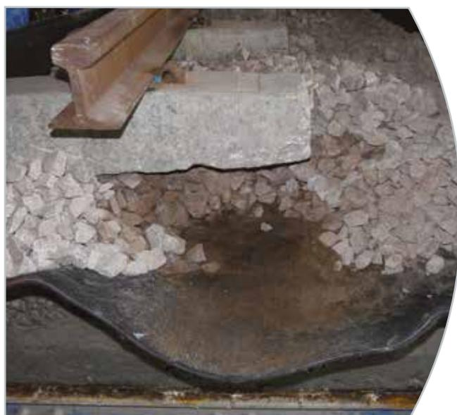
Successful pumping test using TrackTex
