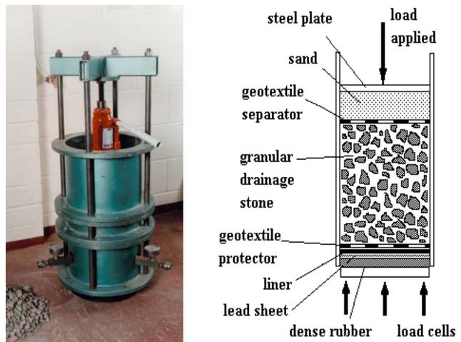
Figure 2: Photo of loaded "cylinder" test and cross section
