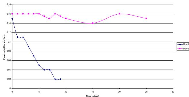
Figure 4: In plane flow results showing rejected Prototype 1 and accepted Prototype 2 with steady state flow
