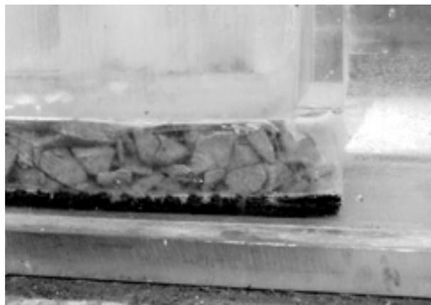
Figure 3: Photo of modified in-plane flow test using stone
