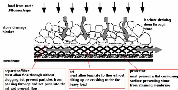
Figure 1: key components and functions of the three main elements of the geocomposite
