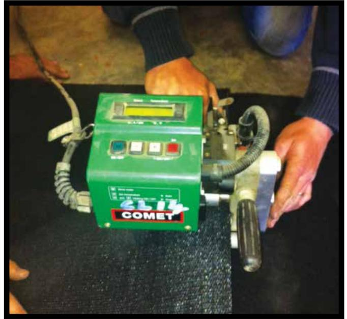
▲ Bonds quickly and easily at roll edges using standard wedge welding equipment.
