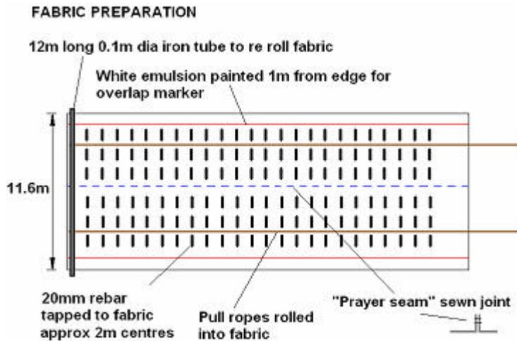
Picture 6c: For deep remote placement. Geotextiles are unrolled remotely using pull ropes which are pre-rolled into a prepared roll. The roll is rolled out sewn to produce wide roll then rebar taped at intervals to the fabric. White markers on the black fabric show the overlap width to the divers at depth.
