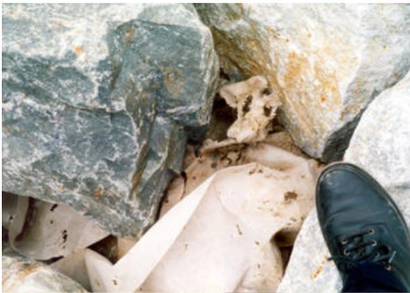
Picture 3: Damage to a thin heat bonded non woven due partially to burst, surface abrasion and lack of cover layer protection
