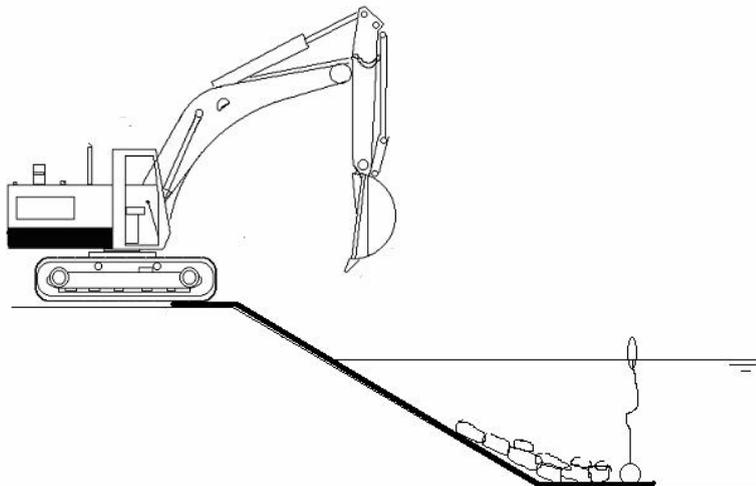
Picture 5a: Trap geotextile with tracks of excavator lower metal pole wrapped in geotextile. Leave pole till fabric weighted by initial stone placement. Retrieve pole by pulling on buoy ropes at ends of pole.
