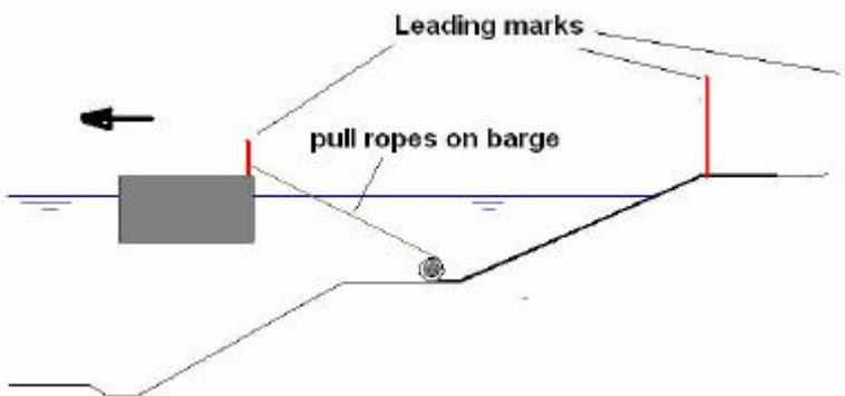
Picture 6a: Longer slopes using steel pole and pre weighted fabric (see preparation below). First slope uses first method then barge takes over handing ropes from shore to barge continues down slope. Additional barge may be used for rock dumping
