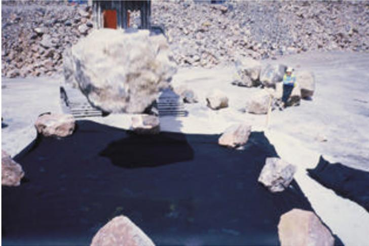
Picture 4: Rock drop test at Cardiff Bay Barrage. Note that fabric is constrained to create “drum” effect likely to occur in worst case on site.
