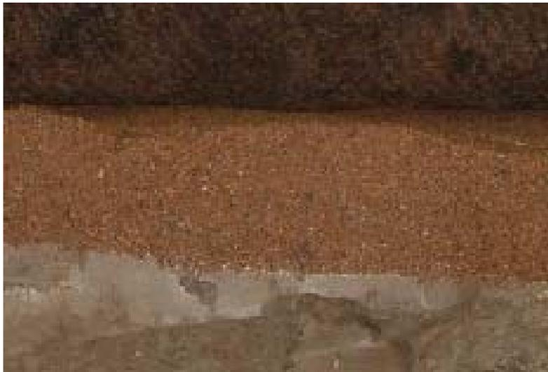
**Figure 7 – Section through geotextile/sand blanket, showing its effectiveness as a separator**
