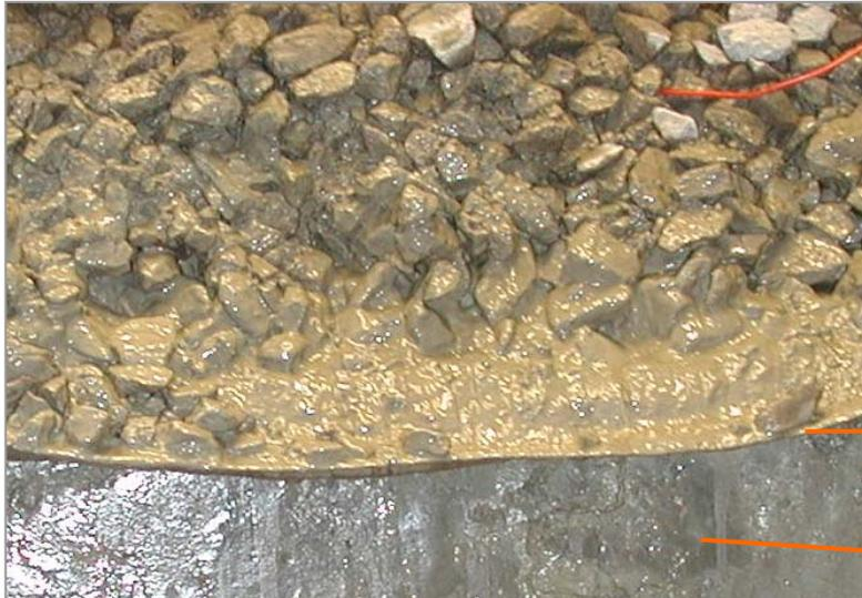
**Figure 5 – generation of clay slurry when using a geotextile alone**
